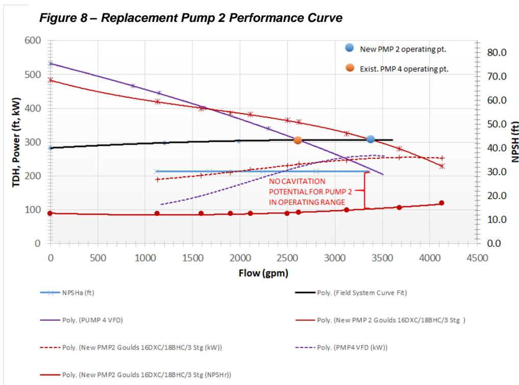
Pump 2’s anticipated performance curves as compared to the performance of Pump 4’s wire-to-water efficiency test results. Equipping Pump 2 with the previously mentioned 3-stage pump ultimately resulted in a decrease in demand of 33.7 kW (434,575 kWh) during the summer months, 26.8 kW average power demand saving over the course of the year, and 725,624 kWh/yr energy consumption savings. The potential rebate and electrical cost savings resulted in less than 1.77 years Return on Investment.
