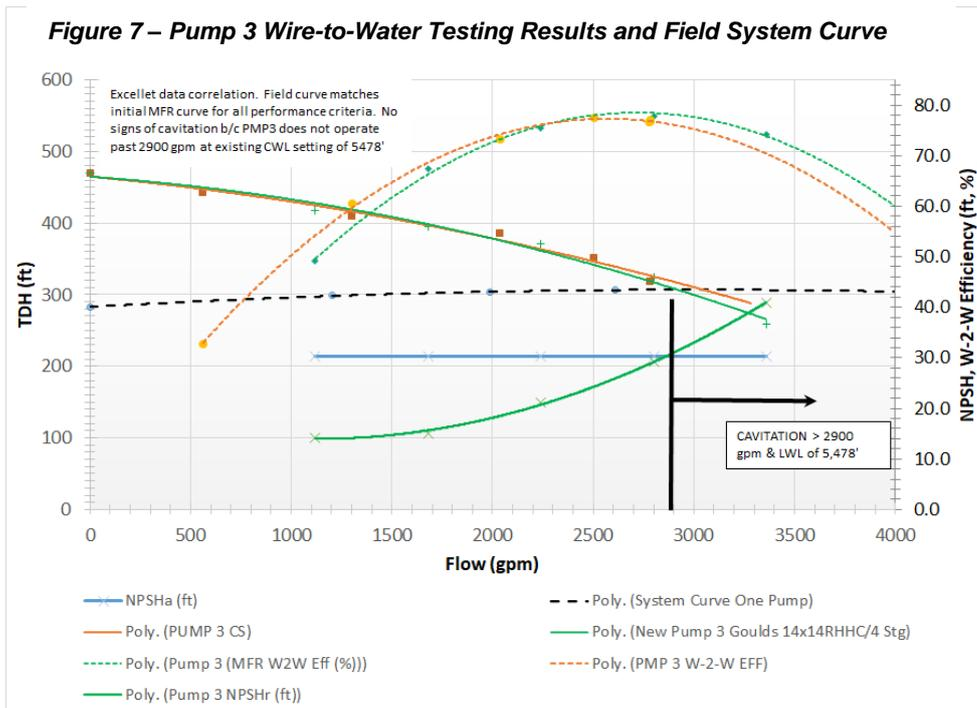
A “low cost” solution was to incorporate all the “no cost” EEMs previously stated, but also replace Pump 2 with a more efficient, lower NPSHR pump. Pump 2 was already scheduled to be equipped with a new 350 hp 3-stage pump with lower NPSHR, that would increase the flow by 800 gpm at 10% less kW than Pump 4 experienced in the field, with no concern of cavitation at the existing water levels. Refer to Figure 8 for
