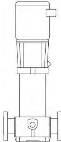
Figure 2.2.9.3.1 — Vertically suspended – in-line casing – multistage diffuser (VS8)
