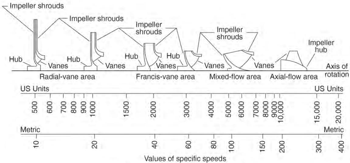
**Figure 1.1.4.1 — General impeller types**
