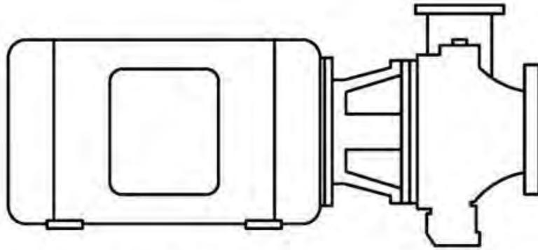
**Pump type OH7: Overhung Impeller, Close-Coupled, Single-Stage, End Suction**
